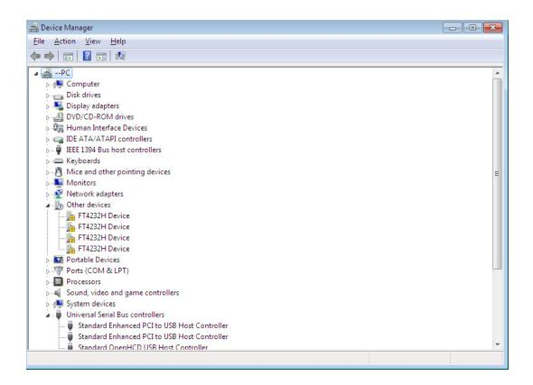
**Step 6:** Right click on the other device to bring up a menu as shown below. From the displayed menu select "Update Driver Software..." This then displays the option for an automatic search or a manual search
