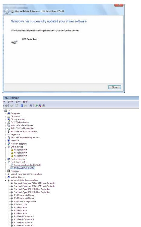
This time the Device Manager does not have an usb <->Serial Port entry under Other Devices but does show entries under Universal Serial Bus Controllers and Ports (COM & LPT). The above screen shot displays a correct installation. The device is now ready to use on COM3.
