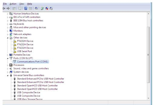
The Device Manager will still show a device under Other Devices but in addition to this there is a new entry under Universal Serial Bus Controllers indicated in the screenshot above as the USB Serial Converter A.
