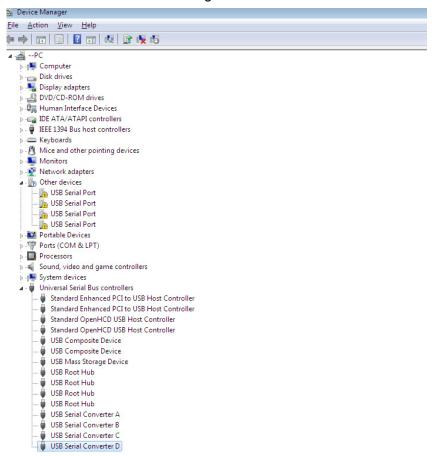
The Device Manager will still show a device under Other Devices but in addition to this there is a new entry under Universal Serial Bus Controllers indicated in the screenshot above as the USB Serial Converter B/C/D.
